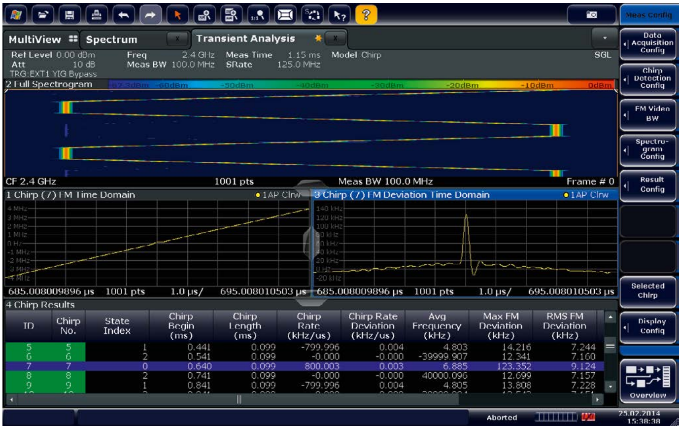
Analysis of a chirp signal with R&S®FSW-K60C. Simultaneous display of spectrogram, chirp rate, chirp rate deviation and summary table.
