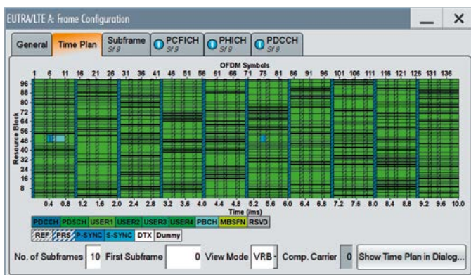
R&S®SMW-K55 LTE time plan example ( download ).
