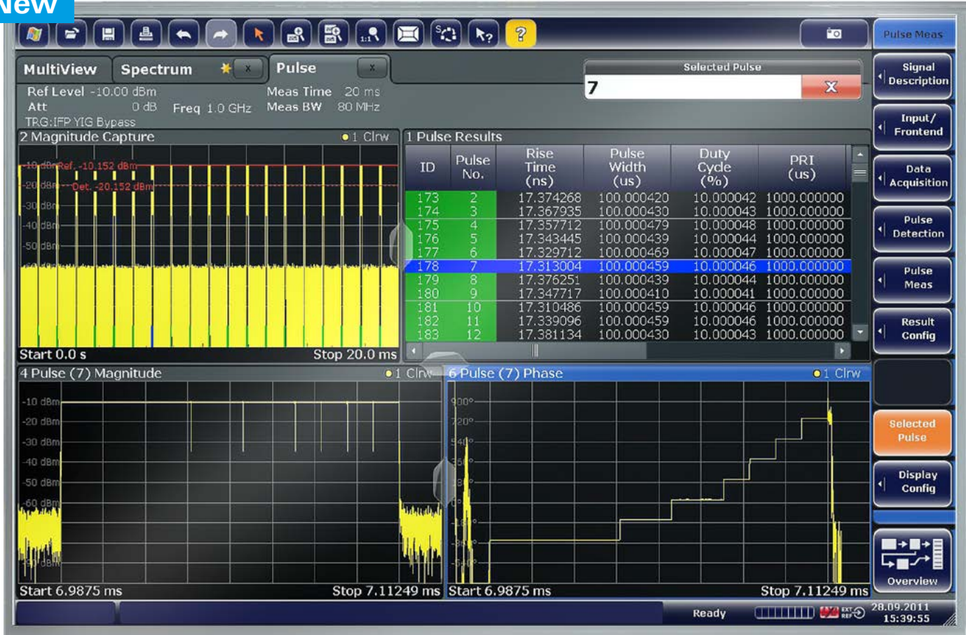
Analysis of a pulse sequence with R&S®FSW-K6.
