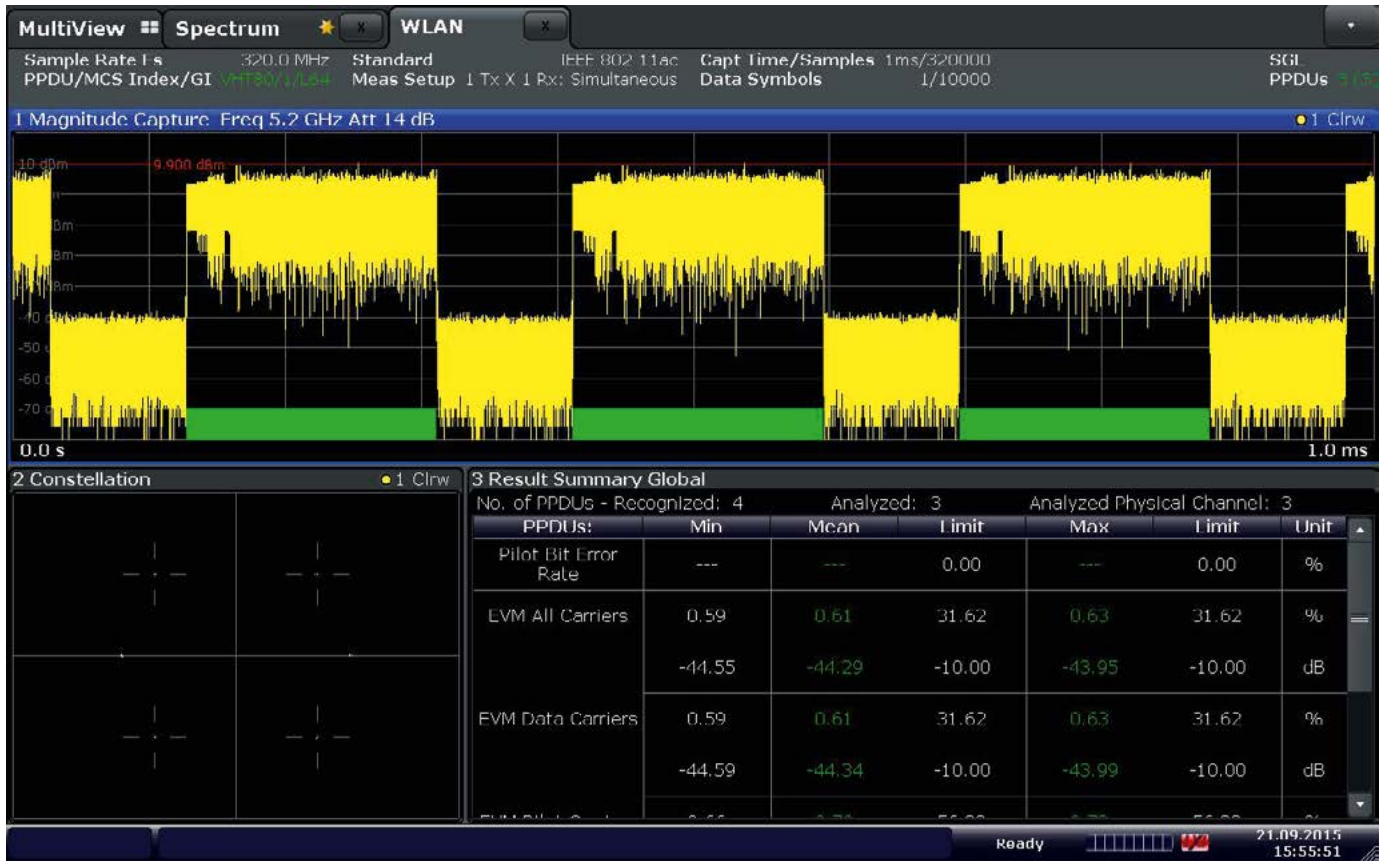
Demodulation of a WLAN 802.11ac signal with R&S®FSW-K91AC.
