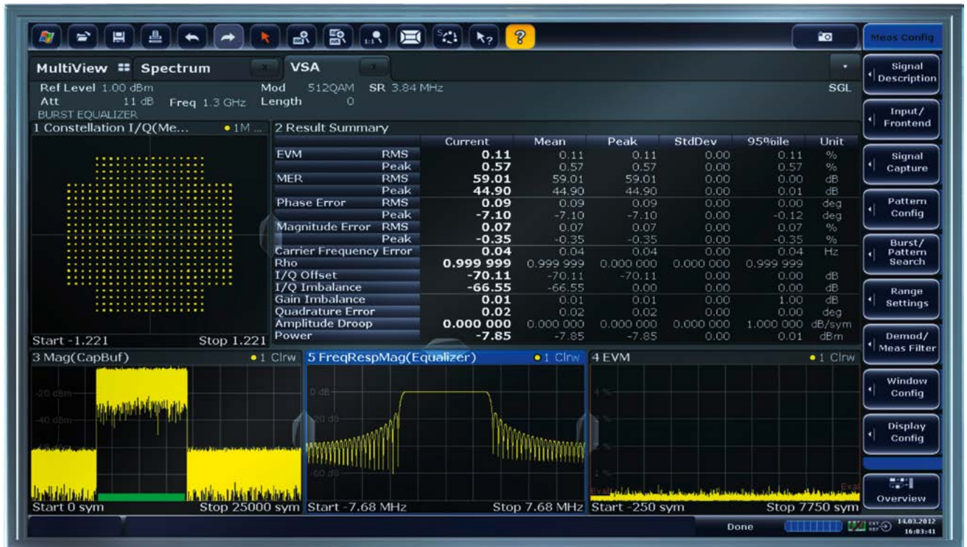
Demodulation of a 512QAM signal with R&amp;S®FSW-K70.
