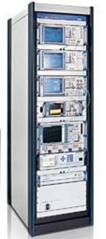
R&S®TS8991 OTA performance test system + R&S®SMBV100A
